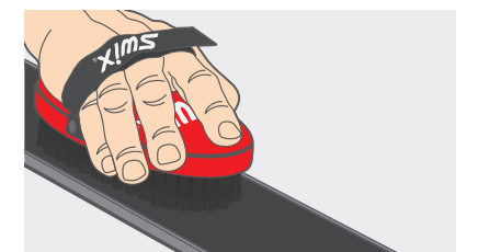
5: Brush firmly with the Steel Brush (T0179 or T0162). The ski is now ready for application of new glide wax.
